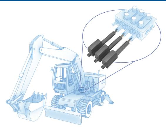
Actuators replace mechanical linkage for spool valve control of boom and tilt cylinders for front end loaders, enabling the use of joystick control.
