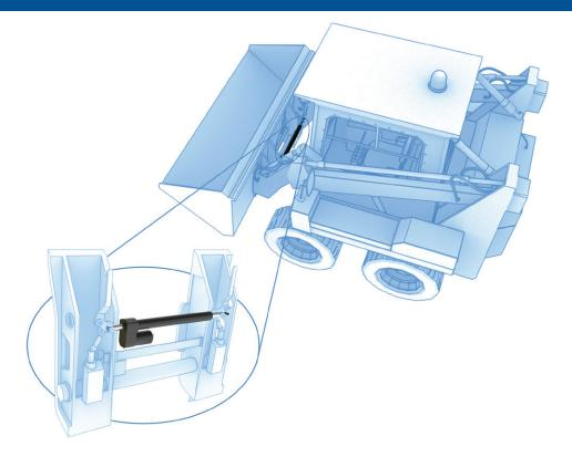
Quick-attach actuators allow the operator to change implements on the loader or skid steer without leaving the seat for improved productivity and safety.
