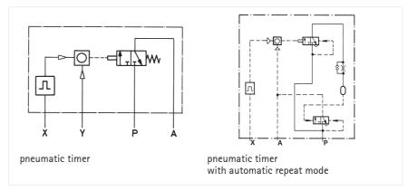
X = air intake timing elementY = pneumatic reset
